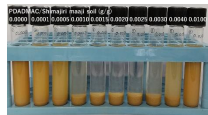
Fig. 1 Photograph of shimajiri maaji soil suspensions with PDADMAC. The weight ratio of PDADMAC to shimajiri maaji soil is shown at a cap.
